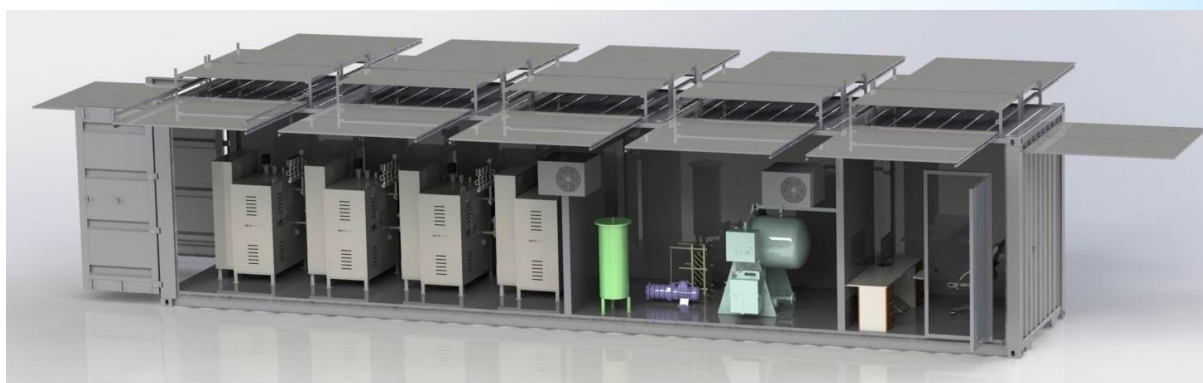
Figure 5 – EMSF container version with biofuel boilers, PV panels and a control workstation
